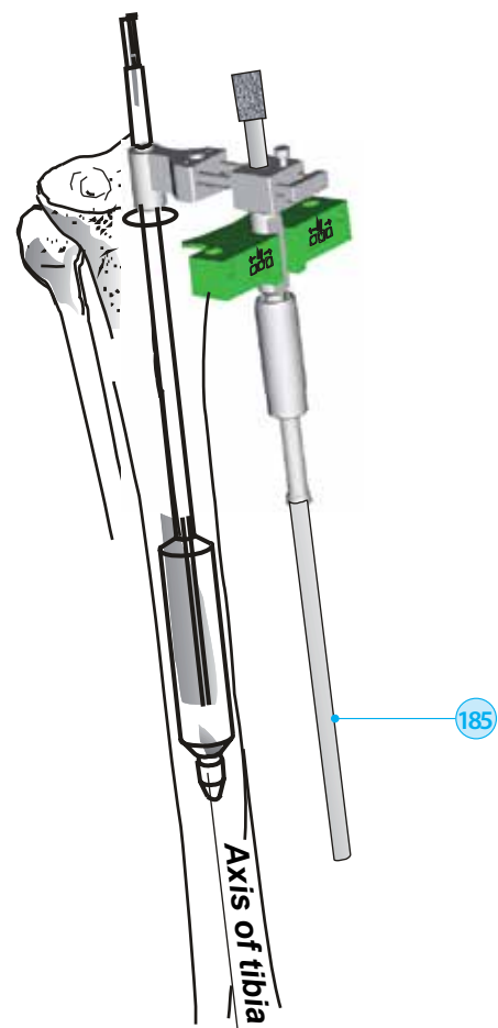
Fig. 8: Assembled intramedullary aiming device and guiding rod with centering rod
